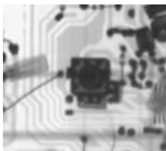
Geometric magnification with microfocus generator
